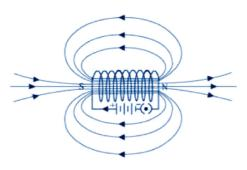
behaves as if it has north pole and south pole. The field lines inside the solenoid are parallel to each other.
