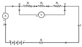
Total/resultant/overall/effective resistance in series  $R = R_1 + R_2 + R_3$
